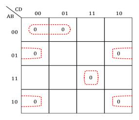
$$F = (A + B + C)(A + \overline{B} + D)(\overline{A} + \overline{B} + \overline{C} + \overline{D})(\overline{A} + B + D)$$
