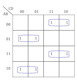
$B3 = \overline{AB}C + \overline{A}B\overline{C} + ABC + A\overline{B}\overline{C} = A \oplus B \oplus C$
